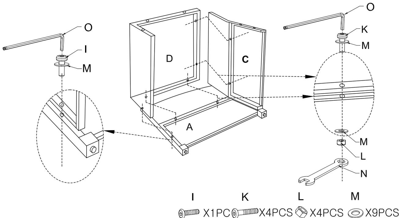
**Step 3.** Attach Right Arm Panel(B) to assembled parts(A,C&D) using Short Bolts (I),Medium Bolts (J),Long Bolts ( K ),Washers ( M ), Nuts ( L ),Wrench ( N ) and Allen Key ( O ) .
