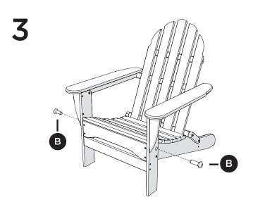
NOTE: Pins can be removed for folding
