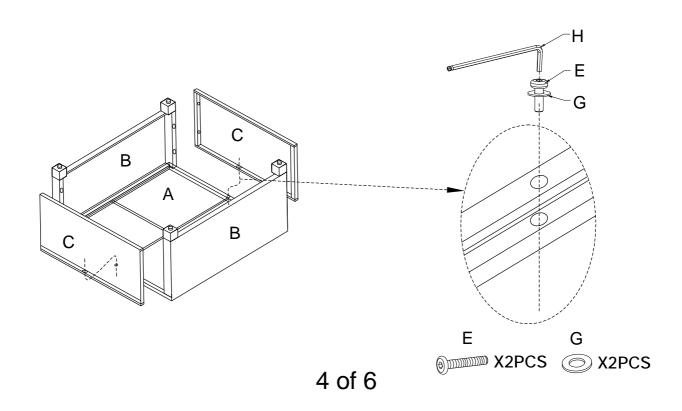
**Step 3**. Attach End Panels (C) to Side Panels (B) using Long Bolts(F), Washers(G) and Allen Key(H).
