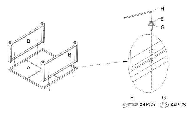
**Step 2**. Attach End Panels (C) to Top Panel (A) using Short Bolts(E), Washers(G) and Allen Key(H).
