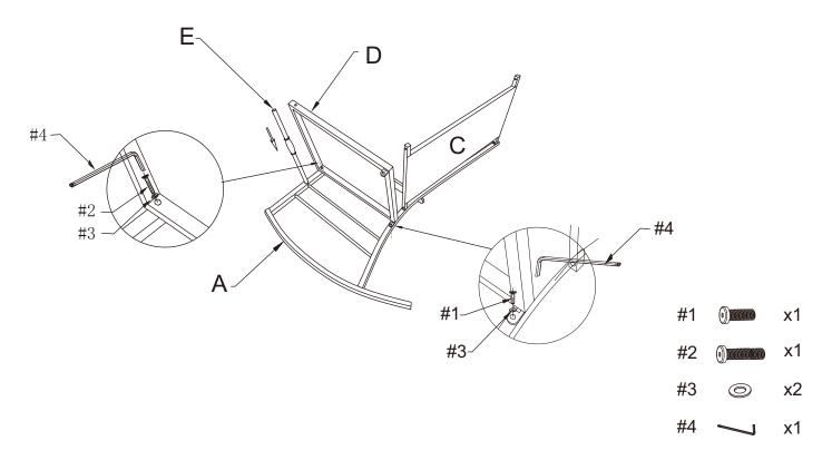
Step 3. Attach left arm panel (part B) to assembled unit (parts A, C, D, & E) using short bolts (part #1), long bolt (part #2), flat washers (part #3) and allen wrench (part #4).
