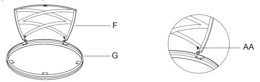
Step 3: Place the Slate Top (E) upside down on a soft place. Put the assembly base over the Slate Top (E) and align bracket, fix by using M6 x12mm bolts (AA). Tighten bolts once they are aligned in all the holes.
