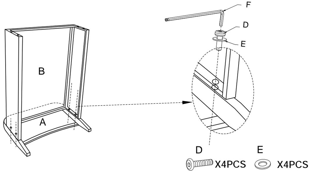
**Step 2.** Attach another Side Panel(A) to Seat Panel(B) using the Bolts(D), Washers(E) & Allen Key (F).
