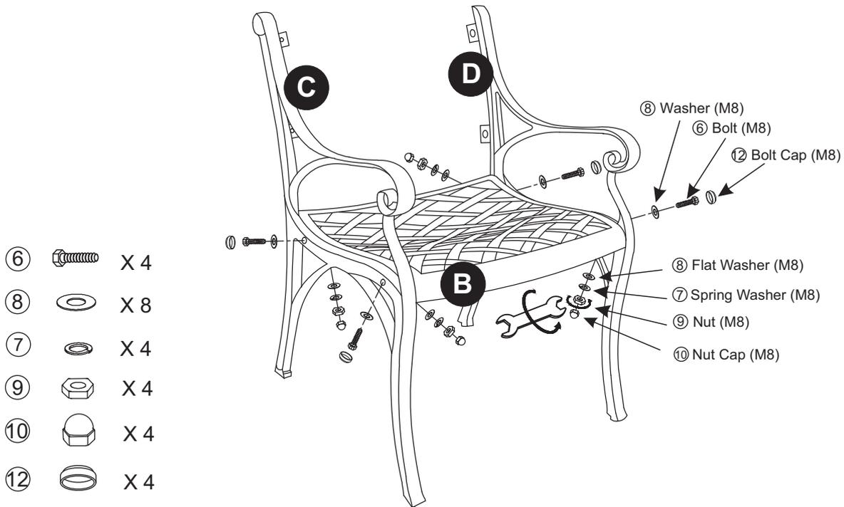
**Step 2: Attach Back (A) to unit with Phillips Head Bolts (Part #1), Flat Washers(Part #3), Spring Washers (Part #2), and Nuts (Part #4). Tighten all bolts of the chair completely. Cover all Nuts with Nut Caps (Part #5).**
