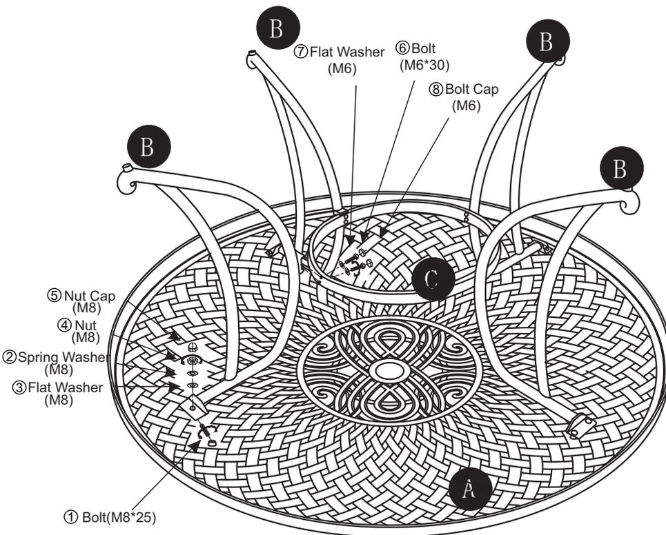
Step 3: Attach Stretcher (C) to attached Legs (B) using Flat Washers (Part #7), and Bolts (Part #6) as shown. Note - Tighten Nuts only half way with wrench (#9). Now attach the other two Legs (B) to Top (A) & Stretcher (C) using the same method as the first two legs. Tighten all bolts completely with wrench (#9).
