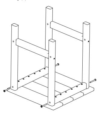
Step 2 Attach braces to sideframes using (4) 2" screws
