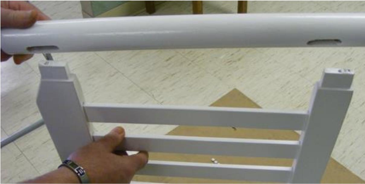
Line up the top of the post with the tenons on the swing back. Press down firmly. Tap with hammer to fully seat.
