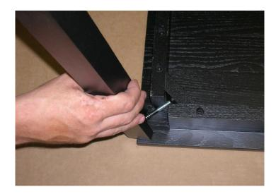
Once all Table Legs (C) are in place begin to attach the Nuts and Washers (B). Start by placing a washer on the bolt first and then thread the nut on finger tight. Complete this for all four corners of the table.
